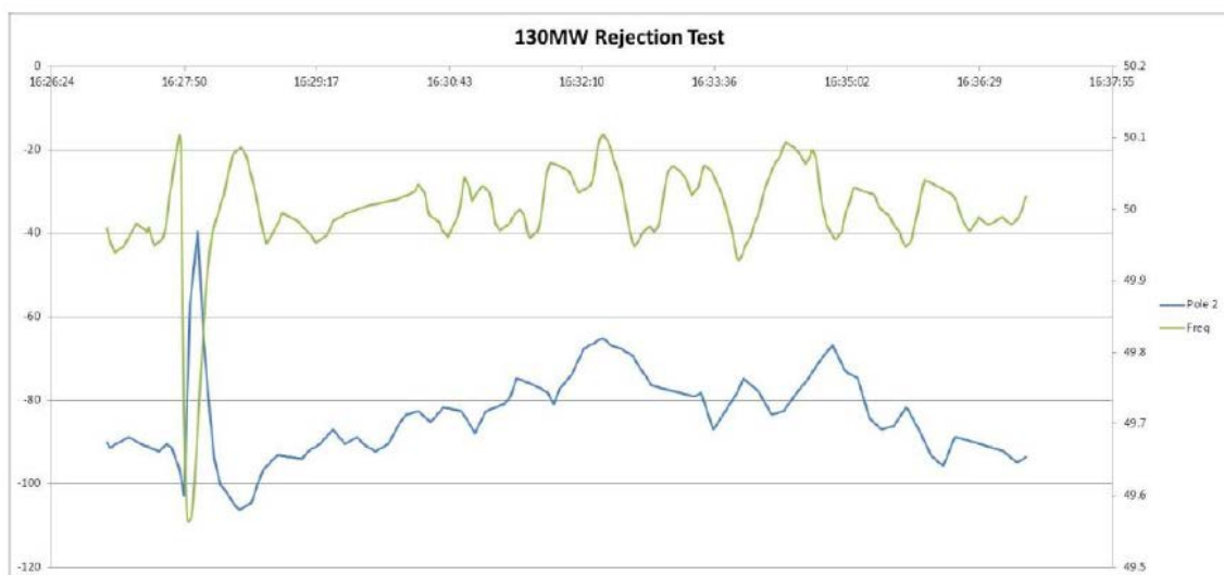
Figure 3 Pole 2 and South Island Frequency responses – 130MW Rejection Test
